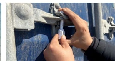
Improved container seal (high security bolt type)
