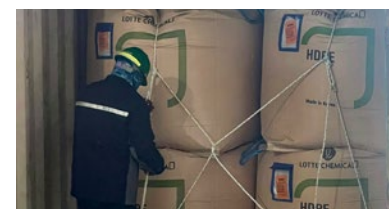
Improved lashing when stuffing containers
